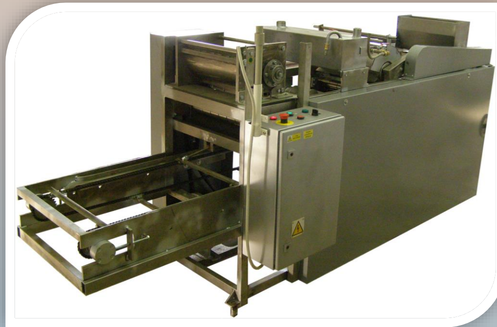
Forming machine with loading on the trays
