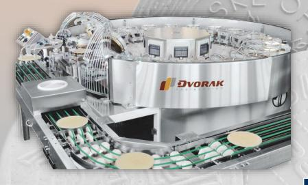
The baking carousel is designed for production of wafer corpuses with a diameter 180-200 mm. This machine has 21 baking plates. The supply of dough on the baking corpuses is realized by pisto pump, the volume of dough is adjustable. An automatic temperature regulation of upper and lower baking plate is possible.
